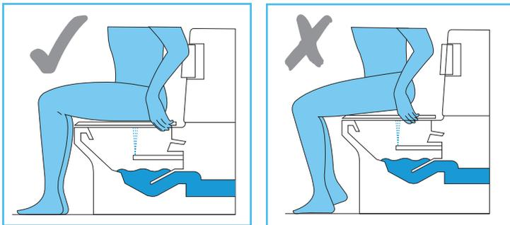
The human anatomy is a major influencing factor, and the shape of the unit should enable the user to sit comfortably with their back supported against the cistern with their torso and legs forming 90° bends. This gives the most appropriate positioning and enables effective bladder and bowel evacuation without undue strain, and ensures correct positioning over the pan/spray, and provides the user with a comfortable and safe sitting position.
